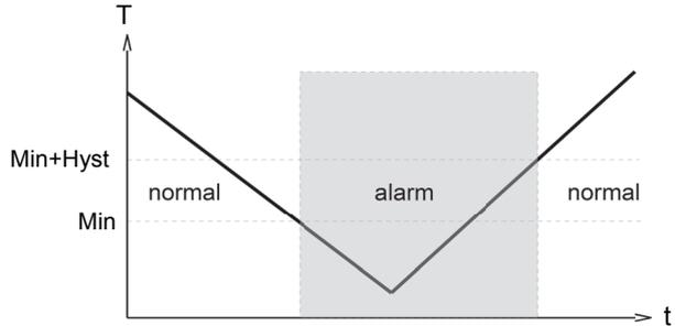
switchover to the alarm state. Return to the normal state occurs when the measured value once more falls below the limit value minus the set hysteresis.
